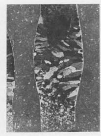
Photomicrograph as seen by Joe Darginis shows a cross section, greatly enlarged, of a weld of two dissimilar metals. Markings indicate grain growth of metal from the heat.
